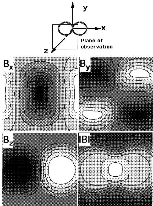
**FIGURE 30.2.** Magnetic field of single-turn figure 8 coil in plane parallel to and one-fourth diameter from the coil:  $x$ ,  $y$ ,  $z$  components and magnitude of field. (From Cohen LG, Roth BJ, Nilsson J, et al. Effects of coil design on delivery of focal magnetic stimulation. Technical considerations. *Electroencephalogr Clin Neurophysiol* 1990;75:350–357, with permission.)
